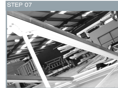
STEP 07 In some situations the vertical drop rod will be attached to a tie bar bracket. Ensure all tie bars are tensioned prior to glazing.
